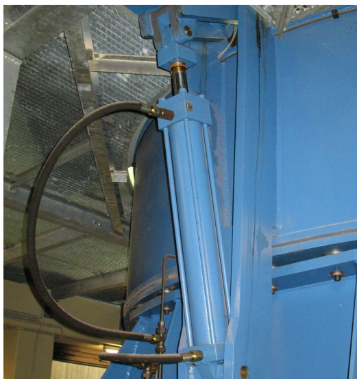
Figure 1: Power element cylinder on a test machine
