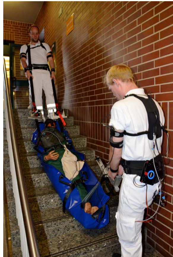
Test arrangement for transport of a patient by means of an evacuation slide sheet
