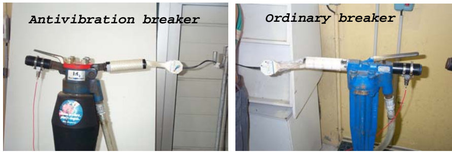
Figure 18: breakers equipped with an accelerometer and the FINGERMAT matrix.
