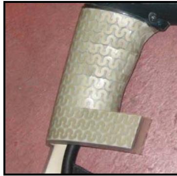
Figura 4. The fingermat wrapped on the driller handle.
