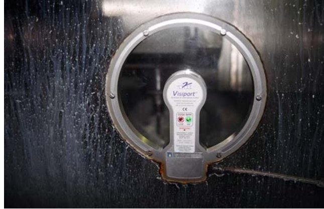
Figure 5: Spin windows to improve visibility in the event of serious contamination with cooling lubricants
