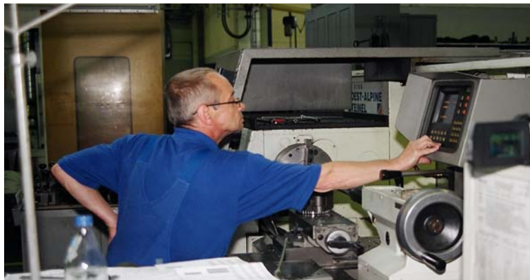
Figure 8: Unfavourable, static upper arm posture from having to reach beyond the arm's range
